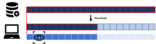
Fig. 2. Progressive Download operation
